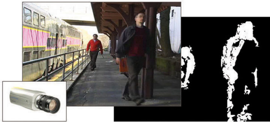
An image captured by Image Acquisition Toolbox (center) from a camera (left), and a display of motion detected by optical flow (right). Callbacks and MATLAB serial I/O capabilities can be used to pan and tilt the camera to track an object.
