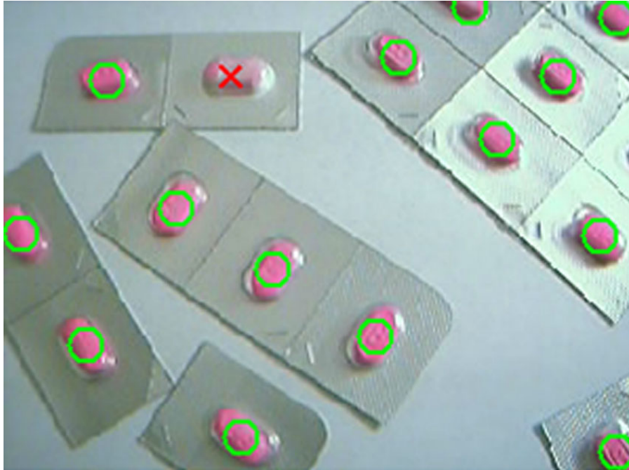
Image of blister packs acquired by Image Acquisition Toolbox. Image Processing Toolbox analyzes the data and marks broken pills.
