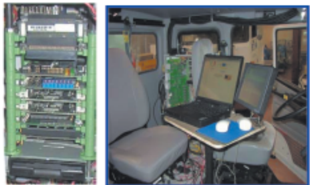
XPC Target stack and vehicle installation.
