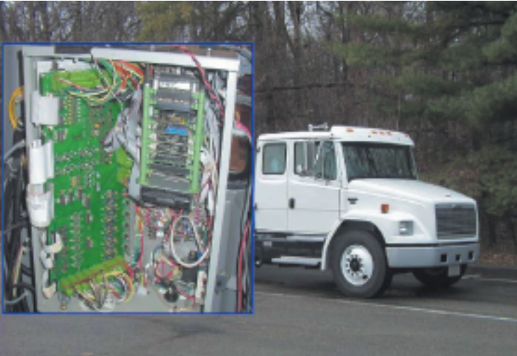
Eaton's prototype medium-duty hybrid truck and system controller.
