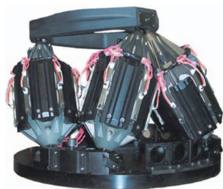
CARCO's six-degrees-of-freedom motion test system.
