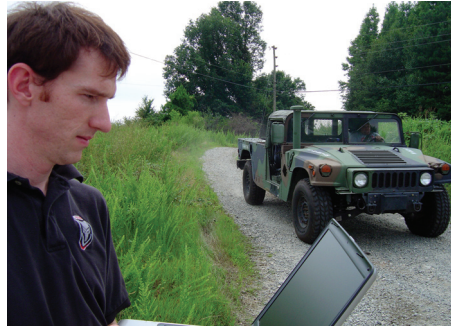
Tuning parameters of a military vehicle's semi-active suspension system with a wireless laptop.
