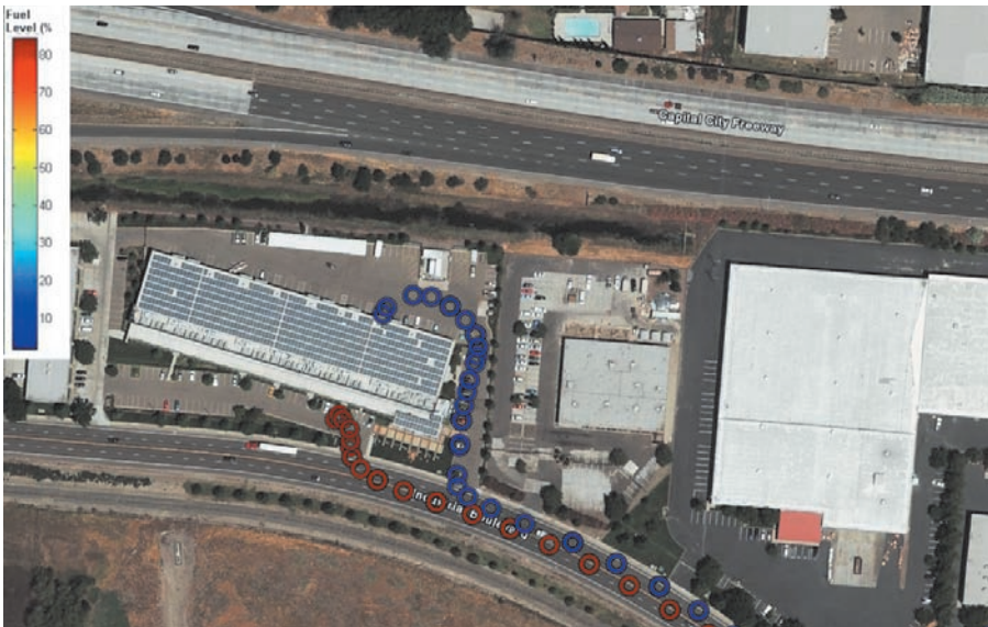
FIGURE 2. Fuel consumption analysis. In this example we see the test car leaving the fueling station with a full tank (red) and returning with a nearly empty tank (blue).
