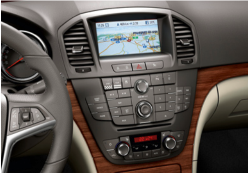
GM vehicle dashboard with the HVAC control system installed.
