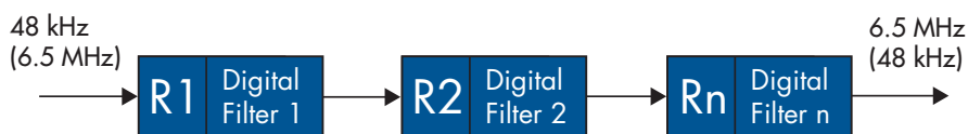
Figure 3. The new design architecture, in which each filter is implemented independently using Filter Design HDL Coder. R1, R2, and Rn represent the rate change (interpolation/decimation) of the first, second, and nth filter in the chain.
