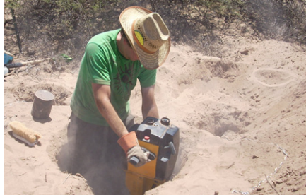
A University of Arizona researcher installing an IRIS broadband seismic sensor to record earthquakes in Argentina.
