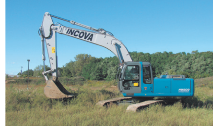
A 25-ton excavator with hydraulic functions controlled by INCOVA’s valve-control system.
