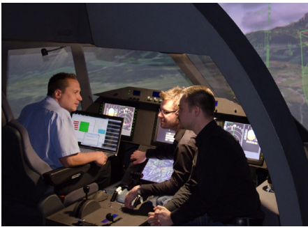
Professor Holzapfel, research fellow Markus Hornauer, and a student test flight control algorithms in the Research Flight Simulator.
