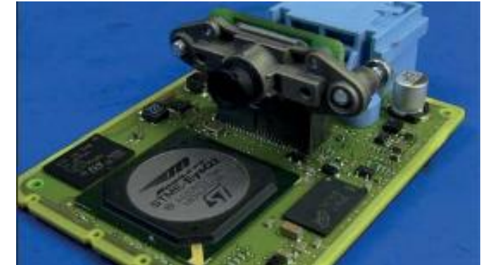
A Mobileye EyeQ2 chip used with a Hyundai lane guidance camera module
