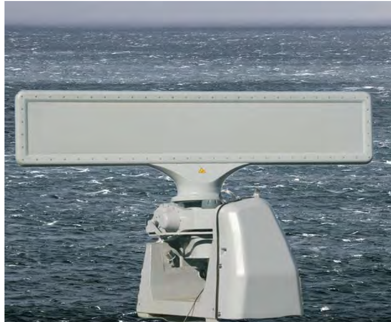
The Reutech RSR 210N multipurpose 2D radar system.
