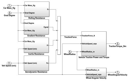
**Simulink Vehicle Traction Model**
