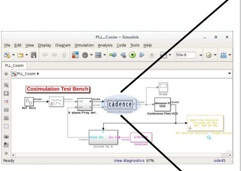
Two variable step solvers working together Charge-pump being simulated in Spectre Rest of the PLL system simulated in Simulink
