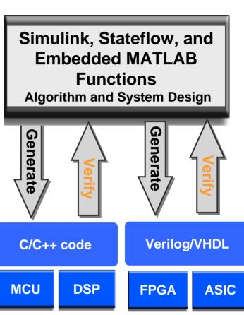
You can verify code on any microprocessor or hardware device.
