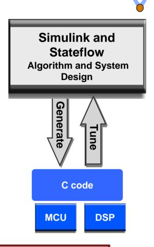
You can deploy code on any microprocessor using Real-Time Workshop Embedded Coder because it generates standard C (ANSI and ISO).
