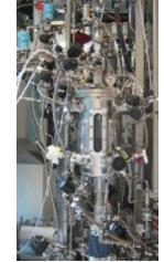
A Genentech microbial pilot plant bioreactor
